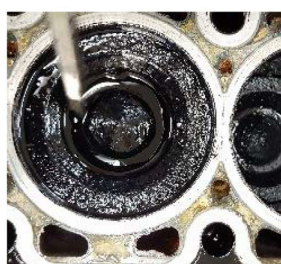
< Engine oil in combustion chamber >
