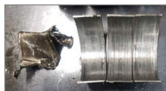
< Connecting rod bearing seizure >
