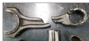
< Connecting rod broken >
